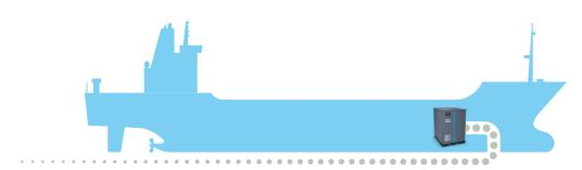
Tiny bubbles below the ship's hull reduce friction to sail faster and lower fuel consumption.
