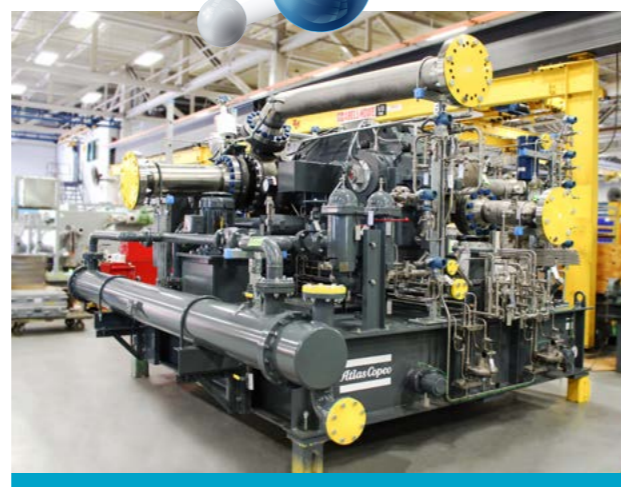
Integrally-g geared centrifugal compressor for oxy-combustion in sCO 2 power cycles.
