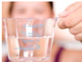
A measuring cup can be used to measure volumes of liquids. This cup measures volume in units of cups, fluid ounces and milliliters.
