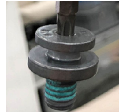
Sockets and bits must grip the bolt/screw to its full gripping area; partial grip without lowered torque, can result in broken bits.
